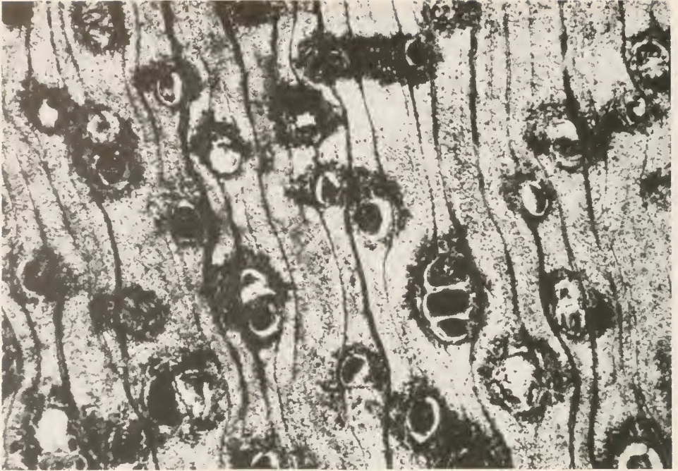
Fig. 5: Cross section. Axial parenchyma vasicentric and partly confluent, vessels with dark contents. \times 50 .
